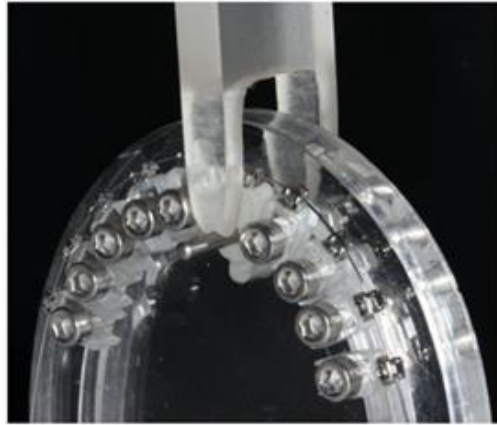
Fig. 3 Clinical simulation device where the central bracket was downward displaced based on the three-point bending output ( -3 mm for GUMMETAL and NiTi and 1.6 mm for SS). The indenter was upward displaced, and the unloading force was recorded until the central bracket reached the initial position
