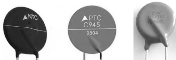
Figura 1. PTC, NTC y varistor
