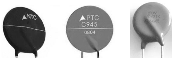
Figura 1. PTC, NTC y varistor
