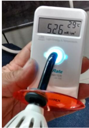
Figura 19. DigiRate Radiometer LM-100 Monitex. LED/Halogen Light Energy & Temperature
